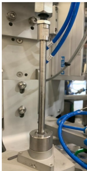
Figure 5-12 The compacting rod
