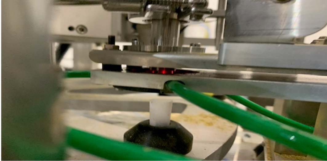
Figure 1 – Optical sensor checking for a paper presence
